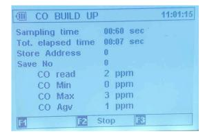
As long as the test has run for longer than 60 seconds the report will be available to Print immediately by pressing the "F1" Key or be saved automatically to the chosen Storage Address for output later.
