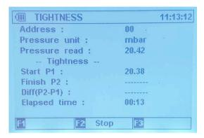
Once the 120 seconds have elapsed the Start, Finish & Difference pressure will be displayed with option for you to Pass or Fail the test at this stage.
