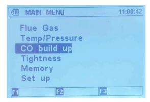
Entering the CO Build Up function will start the Purge Period. During this period you can press the "F2 Key" to skip, if displayed.
