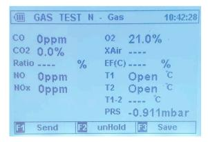
"F1" will send the Held Readings to the Printer, if connected "F3" will allow you to save the Held Readings in the Memory "F2" will unHold the readings and return to Live Readings
