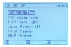
Entering "Mode & Time" will display the following where you can toggle the Display Mode between 7 & 4 Line, adjust the timings for the Let By, Stabilisation & Tightness Pressure Test as well as adjusting the Date & Time
