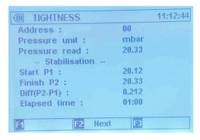
Press the "F2" Key to move onto the Tightness section of the test.
