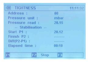
The Stabilisation section of the test will start to count up and complete after 60 seconds.
