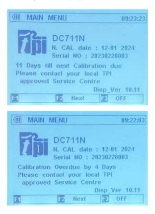
Choosing "Next" will move you onto the Main Menu Screen as displayed below. **Please Note:** In the UK, it is a requirement of BS7967 that an FGA is within calibration and used in conjunction with the manufacturer's instructions therefore it is NOT recommended that "Next" be chosen by the user if the Calibration is Overdue. Doing so will contravene the requirements of BS7967.
