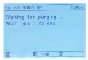
Once the Purge Period is complete the following screen is displayed where you can start the Ambient Air CO Build Up Test.
