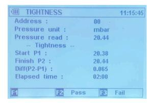
Press the "F3" Key to Fail the test or Press the "F2" Key to finish the test and bring up the Save and Send options. Press the "F2" Key to save the test to the chosen Storage Location.
