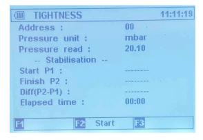
Press the "F2" Key to Start the Stabilisation section of the Test
