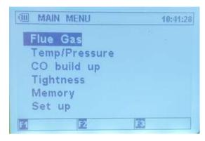
If this is the first time you are turning the DC711 on, we suggest you head over to the "Set-Up" section to investigate the options as described below. Press the Up or Down Arrow Keys, to highlight "Set up" then press the "Enter" key.
