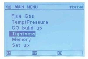
Press the "F1" Key to Zero the pressure, if required, before attaching the pressure hose.
