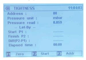
Press the "F2" Key to Start the Test
