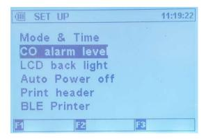
Entering "CO alarm level" will display the following where you can toggle the ambient and High CO alarms On & Off, as well as adjusting the default levels to suit your testing requirements
