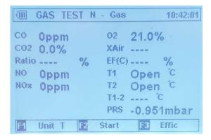
Press the "F1" Key to toggle between Celsius & Fahrenheit or the "F3" Key to cycle through the Efficiency options.
