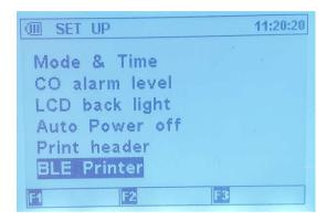
Entering "BLE Printer" will display the following where you can scan and pair available A741BT Bluetooth Printer to your DC711.
