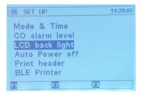
Entering "LCD back light" will display the following where you can adjust the LCD backlight level.
