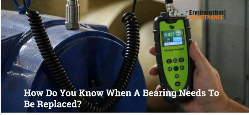
The ISO guidelines for acceptable levels of vibration in rotating machinery form a very good basis for setting alarm levels in the context of Condition Based Maintenance (CBM). These levels can be used to indicate machine status on a "traffic light" basis, e.g. acceptable (green), warning (amber) and critical (red).
